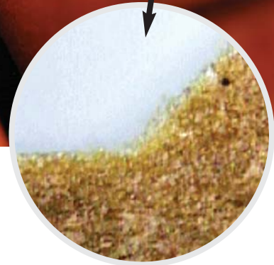
1b) The circled area on right sample illustrates the cleaner lines of the Uni-sanded profile and the more even and economically painted surface.
