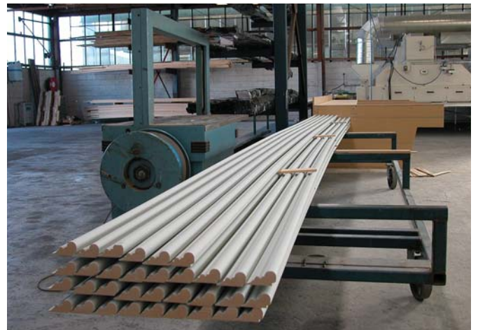
Moulding after sanding and painting.
